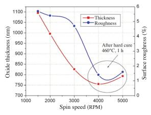
FIGURE 6. Characteristics of SOG by spin speed variation
