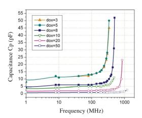
FIGURE 7. Parasitic capacitance vs. frequency for various oxide thickness
