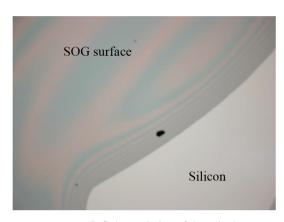
FIGURE 5. Color variation of deposited SOG layer
