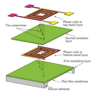
FIGURE 1. Schematic configuration of coupled coil structure
