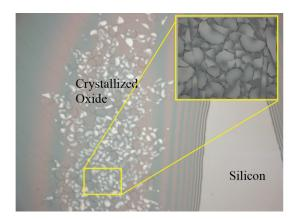
FIGURE 3. Microphotograph of crack building due to the thermal stress
