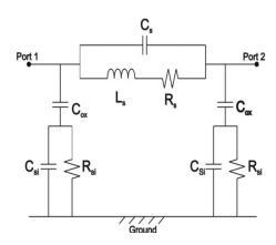
FIGURE 2. Simplified Pi-lumped element circuit model of a spiral coil
