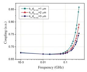
FIGURE 8. Coupling characteristics as a function of oxide thickness between metal and substrate, N = 3, w = 100 micrometers, s = 50 micrometers
