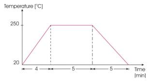
FIGURE 4. Temperature ramping profile in baking procedure of SOG layer
